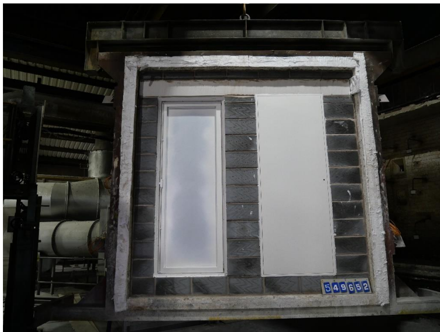
Figure 17 Exposed face of the specimens before the start of the test
